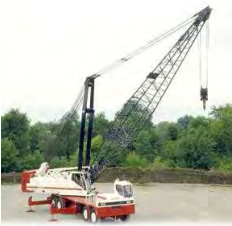
Figure 12.3. 200-ton capacity lattice-boom crane manufactured at the Link-Belt facility in Lexington, one of many crane models produced. Courtesy Link-Belt Construction Equipment Company.
